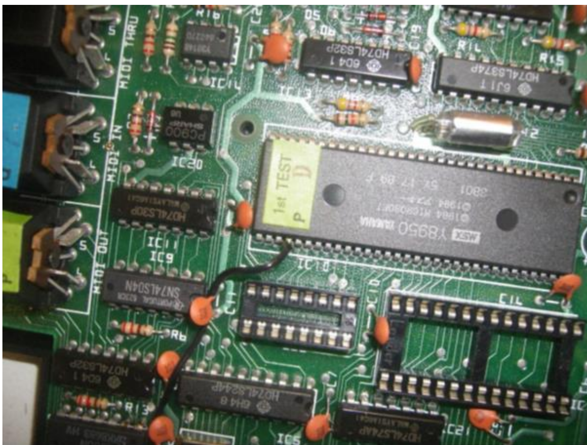
The black wire connecting pin 35 of IC10 to pin 9 of IC2.
