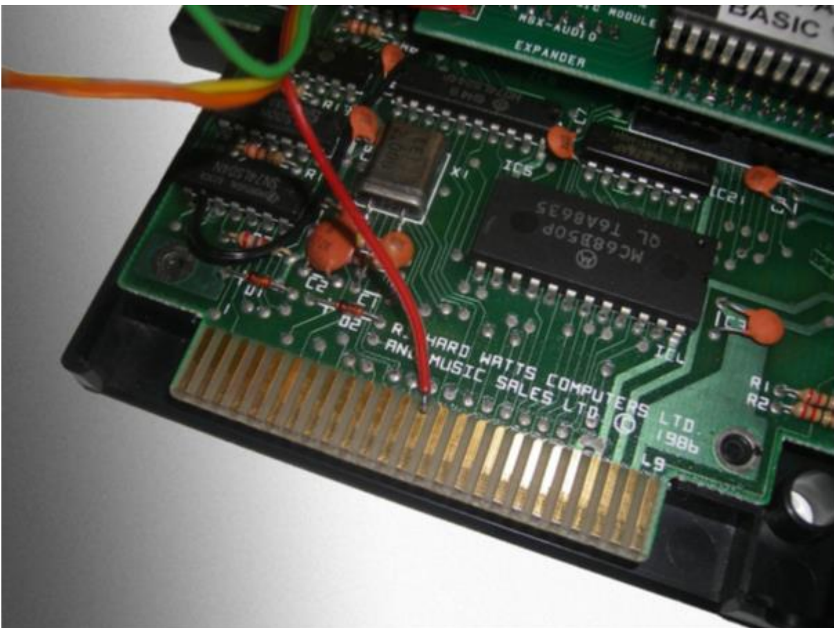
The red wire connected to pin 25 of the slot connector.
